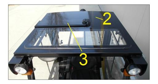
2. Put the roof (2) on the of OHG and place the following passage for access to batteries (3). Put the lateral gap equal.
