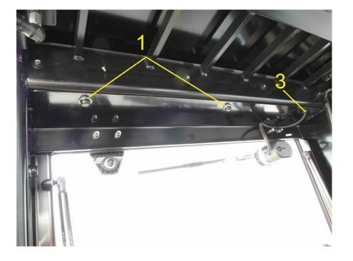
3. Put the rear panel between the rear profiles of the OHG and screw it with 2 screws HM10x25 and 2 screws M8x20
