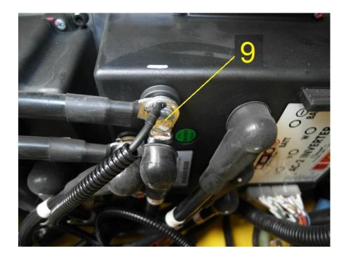
Connect the negative wire of heater electric bundle on point (9)
