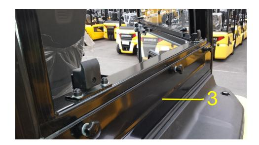
5. Seal marked edges using silicone
