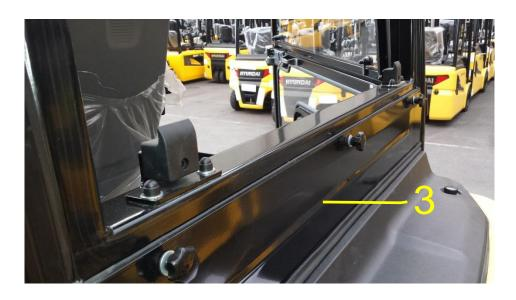
5. Seal marked edges using silicone
