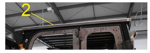
2. Put the roof (2) on the of OHG. Put the lateral gap equal.
