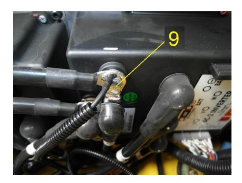
8. Connect the negative wire of heater electric bundle on point (9)
