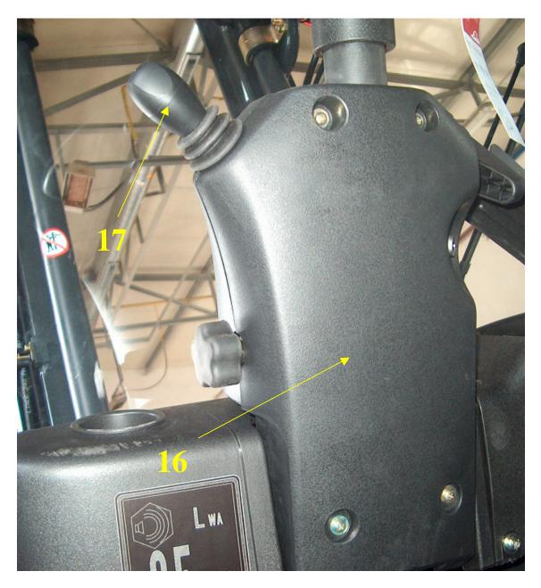
18. Remove the blank plug, and attach the windshield wiper (16); Attach the wiper arm and blade (18).
