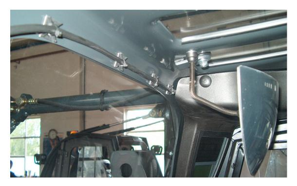
14. Screw down the side and top mask covers.15. Lead the cables to (15) front working lights, driving lights, windshield wiper and to the heater.
